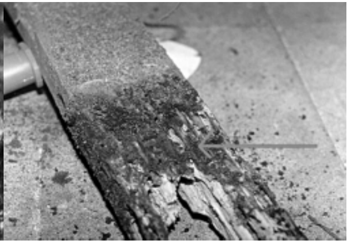
Wood damaged by Reticulitermes lucifugus
